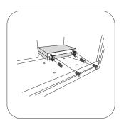
You can put one HDD/SDD below the bracket and one above the bracket.
