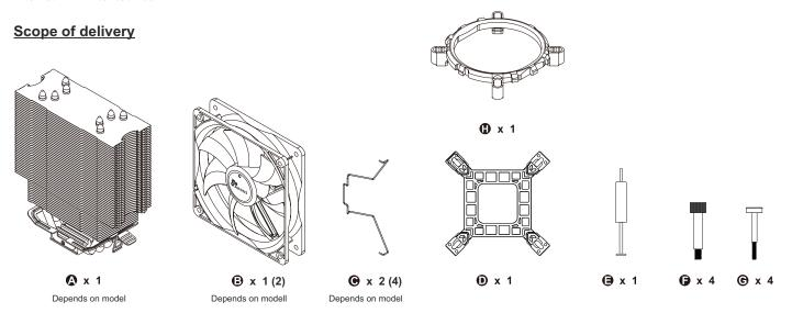
The included socket adapter D is for Intel-Socket 775/ 1150/ 1151/ 1155/ 1156/ 1200/ 1366 mounting. There's no adapter necessary for mounting on AMD-Socket FM2+/ FM2/ FM1/ AM4/ AM3+/ AM3/ AM2+/ AM2. This cooler won't fit on any other socket as those mentioned before.
