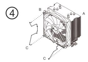
Fix the fan B with brackets C at cooler A (SU-280 has a fan on both sides).
