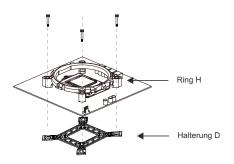
Place the back plate D behind the mainboard and fix it with screws through the ring H. Some mainboards have the back plate already installed. In this case you dont need the back plate D.
