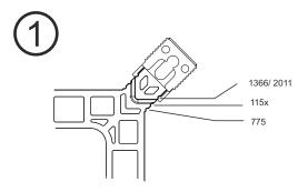
Adjust all brackets on the back plate D depending your CPU socket.
