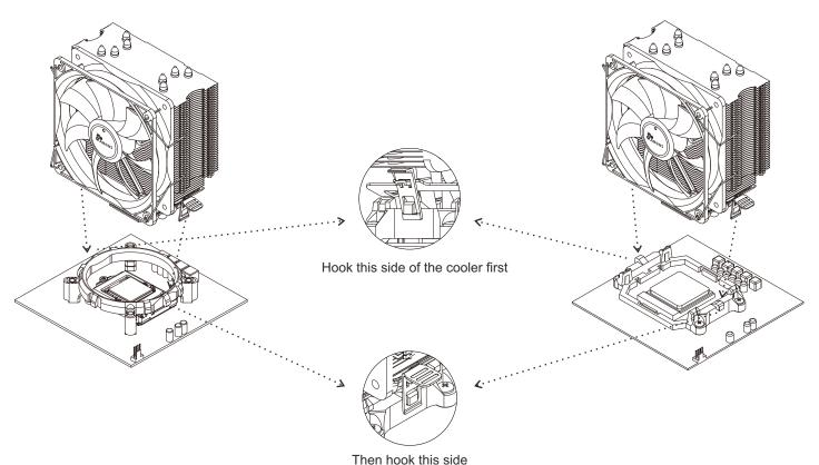
At last connect the 4pin plug of the cooler with the according socket on your mainboard. Please read also the manual of the mainboard. The installation is complete now.
